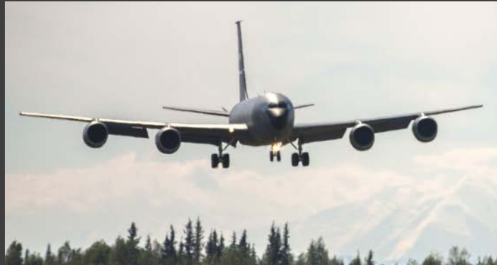
KC-135 Stratotanker: A military aerial refueling aircraft with a crew of three. It provides aerial refueling support to Air Force, Navy, Marine Corps and allied nation aircraft and is capable of transporting litter and ambulatory patients using patient support pallets during aeromedical evacuations.
