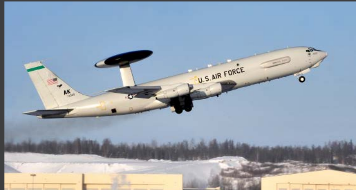
E-3 Sentry: An airborne warning and control system, or AWACS, aircraft with an integrated command and control battle management, surveillance, target detection, and tracking platform. It is a modified Boeing 707/320 commercial airframe with a rotating radar dome.
