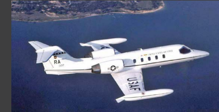
C-21: A twin turbofan-engine aircraft used for passenger and cargo airlift. The aircraft can transport one litter or five ambulatory patients for aeromedical evacuation operations. It has a crew of two and can carry eight passengers and 42 cubic feet of cargo. The C-21 is the military version of the Learjet 35A business jet. (USAF 2019)
