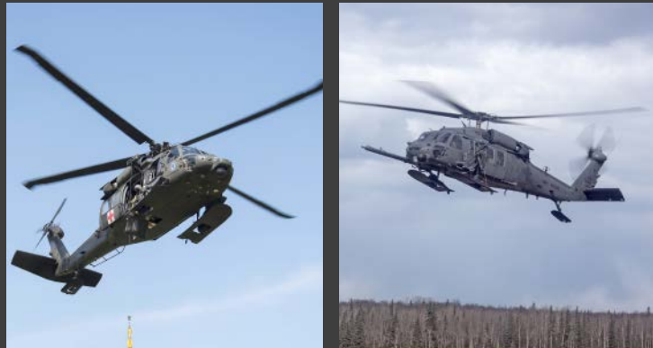
UH/HH-60: The UH-60 Black Hawk is a twin-engine, medium-lift helicopter that provides air assault, general support, aero-medical evacuation, command and control, and special operations support to combat and stability operations. An 11-person, fully-equipped infantry squad can be lifted in a single Black Hawk. The Sikorsky MH060G Pave Hawk is a twin-turboshaft engine helicopter in service with the Air Force. It is a derivative of the UH-60 Black Hawk and incorporates the Air Force's PAVE electronic systems program.
