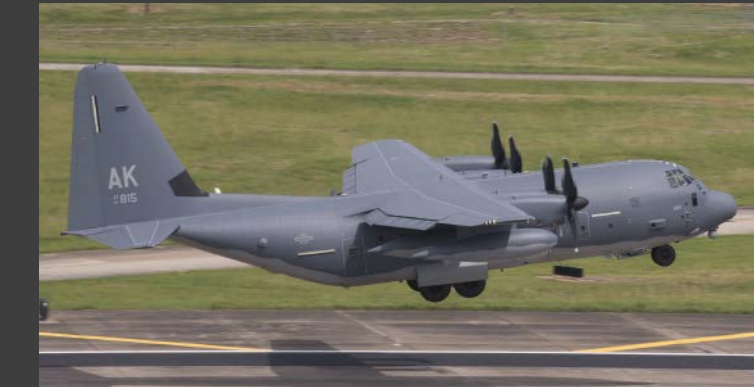
HC-130J Combat King II: A version of the well-known C-130 Hercules tactical transport aircraft that has been specially modified and upgraded to perform combat search-and-rescue missions. The HC-130J supports missions in all-weather and geographic environments. It is also tasked for airdrop, helicopter air-to-air refueling, and forward-area ground refueling missions and can also support humanitarian aid operations, disaster response, security cooperation/aviation advisory, and evacuation operations.
