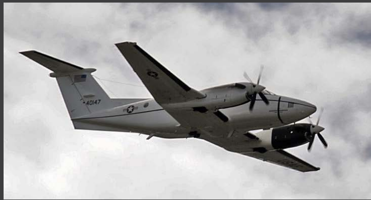
C-12F Huron: A twin turboprop aircraft that provides operational support airlift of passengers and cargo. The C-12 has a crew of two and can carry up to eight passengers. The aircraft has a cargo capacity of 56 cubic feet. The C-12 can also transport patients on medical evacuation litters.
