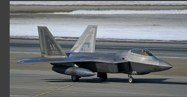
F-22 Raptor: A fifth-generation, single-seat, twin-engine, all-weather stealth tactical fighter aircraft. The F-22 performs both air-to-air and air-to-ground missions and is a critical component of the Global Strike Task Force.
