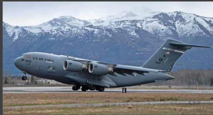
C-17 Globemaster III: A cargo aircraft capable of rapid, strategic delivery of troops and all types of cargo to main operating bases or directly to forward bases in the deployment area. The maximum payload capacity of the C-17 is 170,900 pounds, and it has an approximate cruise speed of 450 knots. The aircraft is operated by a crew of three: a pilot, co-pilot, and loadmaster.
